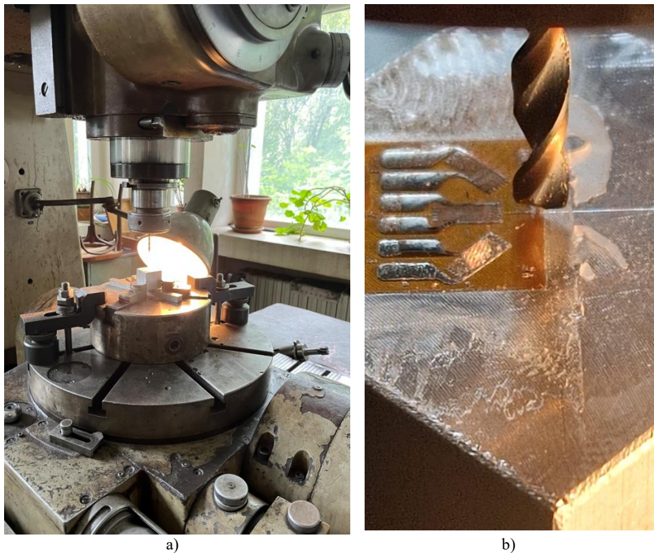
Fig. 5. Drilling the hole: general view (a); approaching the drill to the cube (b)
