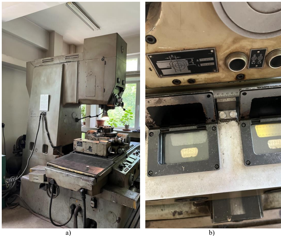
Fig. 3. Coordinate drilling machine (a) and position display with accuracy of \pm 1\mu\text{m} (b).
