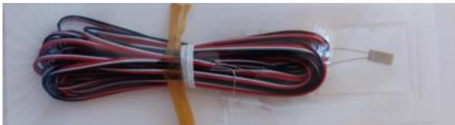
Fig. 6. Strain gauge type MM-Vishay C2A-06-125LW-120, with pre-attached wires.
