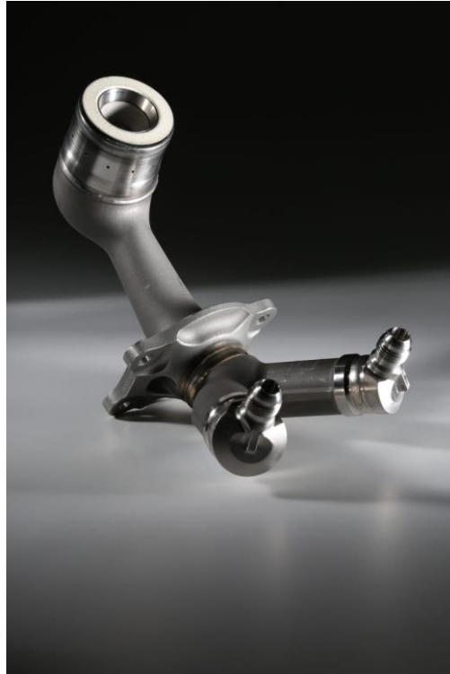
Fig. 3. GE Aviation fuel injector for the LEAP engine, consolidated from 20 parts into a single 3D-printed component (GE Additive_Path to Production_White paper_Final.pdf)
