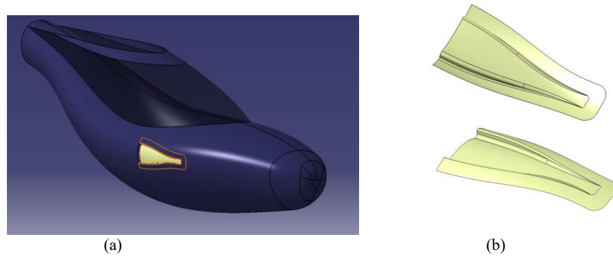
Fig. 2. NACA intake a) position on fuselage; b) 3D model of NACA intake
