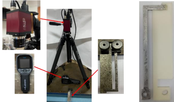
Fig. 5. Experimental set-up and the investigated actuator made of two different materials.
