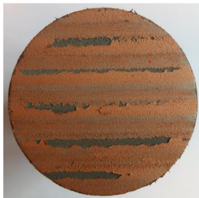
Fig. 24. Fracture after bond strength test [92].
