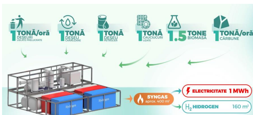
Fig. 10. Molecular disintegration technological flow. Source: www.wpowertech.ro
