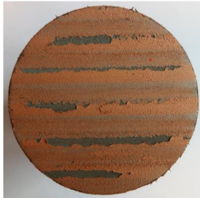
Fig. 24. Fracture after bond strength test [92].
