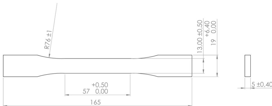
Fig. 1. Specifications of tensile sample.
