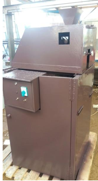
Fig. 4. Differential magnetic separator with controllable magnetic fields.
