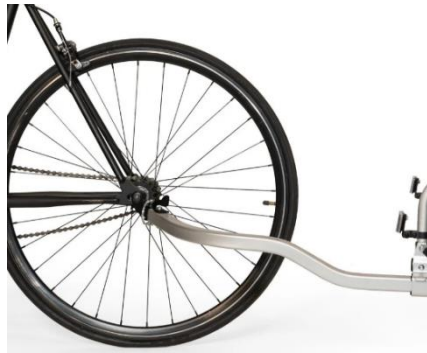
Fig. 4. Attachment of the trailer on the rear wheel axle [10].
