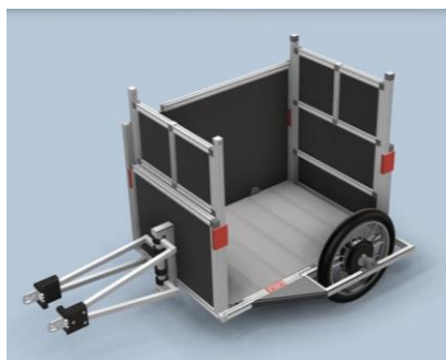
Fig. 18. Renderings for the final assembly design of the attachment in the setting for minimum height and length.
