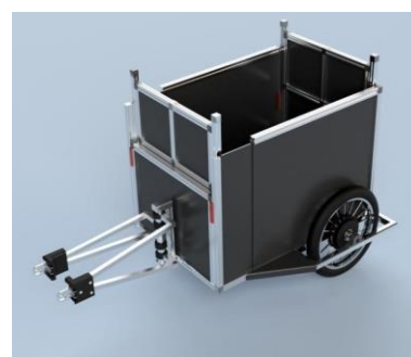
Fig. 18. Renderings for the final assembly design of the attachment in the setting for minimum height and length.
