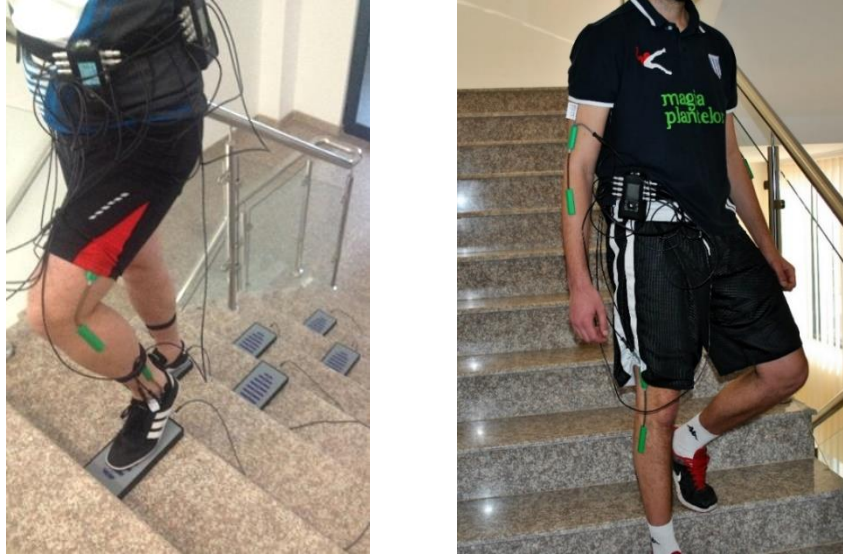
Fig. 3. The equipment mounted on a subject during ascending and descending the stairs.
