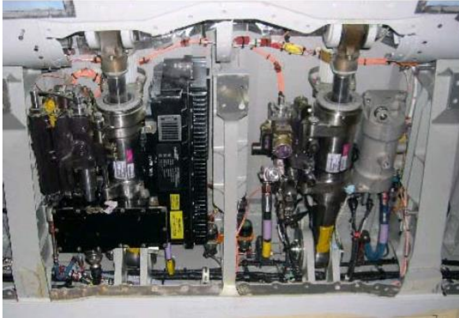
Fig. 10. A pair of EHA and EHSA used on the horizontal stabilizer of A380 [12]
