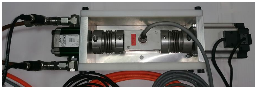
Fig. 21. Pumping assembly including the pump, the servomotor and the torque-speed transducer.
