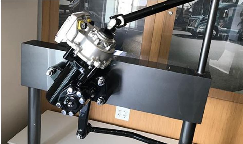
Fig. 14. Complex hybrid steering system for autonomous driving [15]
