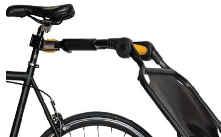
Fig. 5. Attachment of the trailer on the seat post [9].
