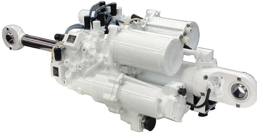
Fig. 8. Redundant EHA for the tail of F35 [11]
