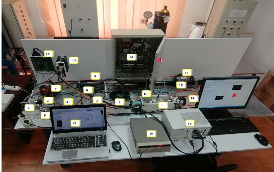
Fig. 20. Overall view of the test bench: 1 – gear pump with motor, torque-speed transducer; 2 – pressure transducers; 3 – block of pressure limiting valves; 4 – releasable directional valve; 5 – check valve; 6 – valve for charging the system with oil; 7 – hydropneumatic accumulator; 8 – hydraulic cylinder with mass and elastic load; 9 – position transducer; 10 – torque and speed adapter; 11 – interface of the torque and speed transducer; 12 – signal converters and power supply; 13 – brushless motor driver; 14 – brushless motor; 15 – AD interface; 16 – PXI digital controller for position loop; 17 – data acquisition system; 18 – mass and elastic load; 19 – functions generator.
