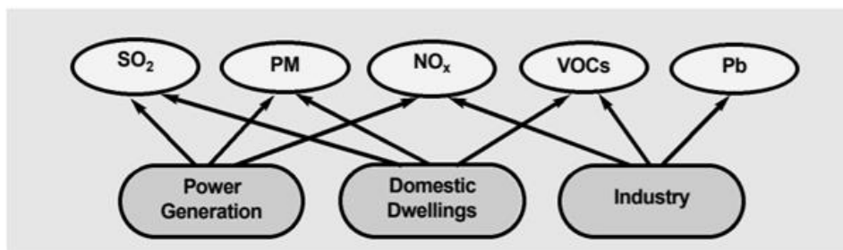
Fig. 2. The main atmospheric pollutants from stationary sources [19]: SO 2 (sulfur dioxide); PM (particulate matter); NO x (nitrogen oxides); VOCs (volatile organic compounds); Pb (lead).
