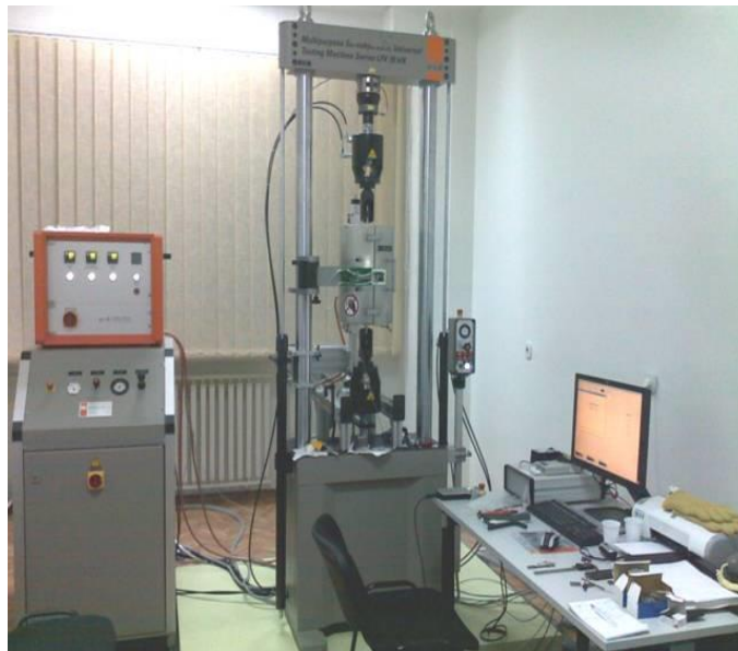
Fig. 4.1. Instrumented Walter+Bai mechanical testing machine for the acquisition and highlighting of fatigue characteristics.
