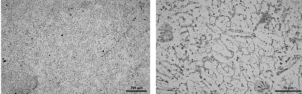
Fig. 4.3. The microstructure of the etched C (7.5% ZrB<sub>2</sub>) composite, at different magnifications.
