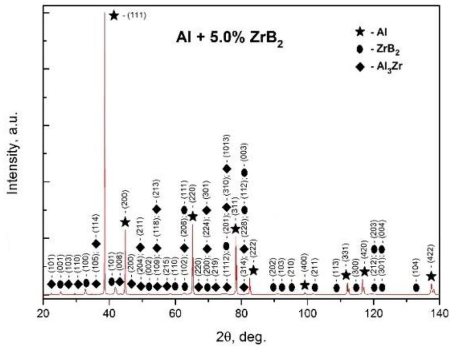
Fig. 4.10. XRD patterns of AA 6063/5% ZrB<sub>2</sub> composites after 10 min of reaction time.
