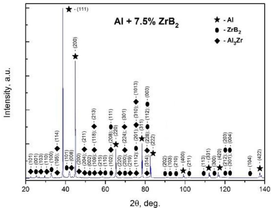
Fig. 4.11. XRD patterns of AA 6063/7.5% ZrB<sub>2</sub> composites after 10 min of reaction time.
