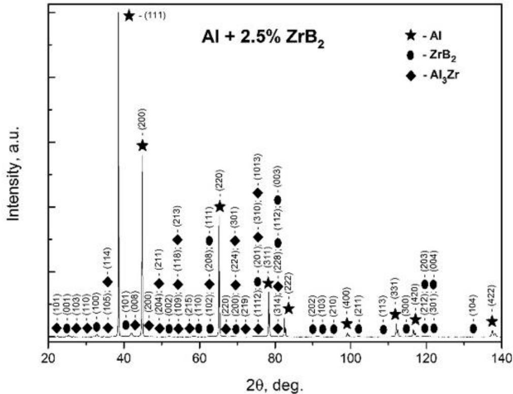
Fig. 4.9. XRD patterns of AA 6063/2.5% ZrB<sub>2</sub> composites after 10 min of reaction time.
