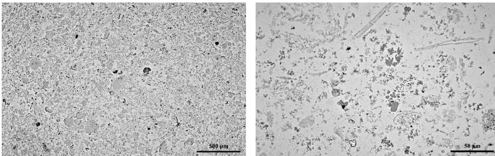
Fig. 4.4. The microstructure of the etched C (10.0% ZrB<sub>2</sub>) composite, at different magnifications.
