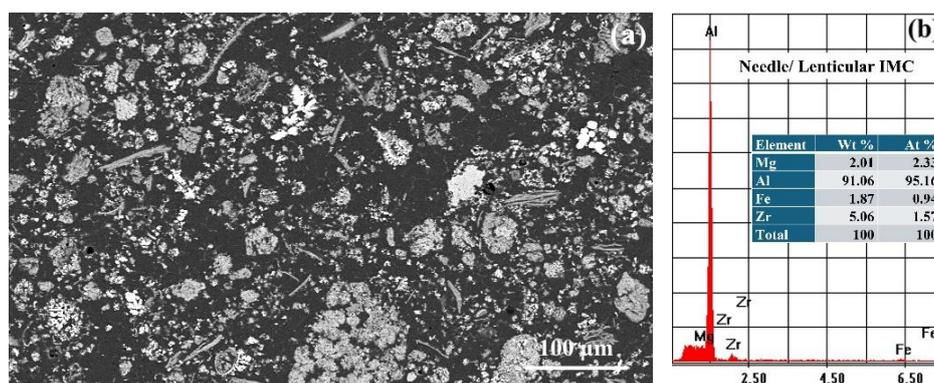
Fig. 4.8. SEM image (a) and EDS analysis of AA6063/ZrB<sub>2</sub> IMC (b) with 10.0% ZrB<sub>2</sub>.
