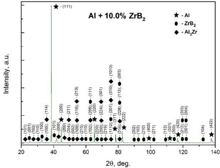
Fig. 4.12. XRD patterns of AA 6063/10% ZrB<sub>2</sub> composites after 10 min of reaction time.
