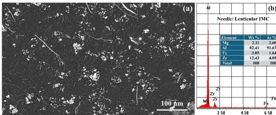
Fig. 4.5. SEM image (a) and EDS analysis of AA6063/ZrB<sub>2</sub> IMC (b) with 2.5% ZrB<sub>2</sub>.
