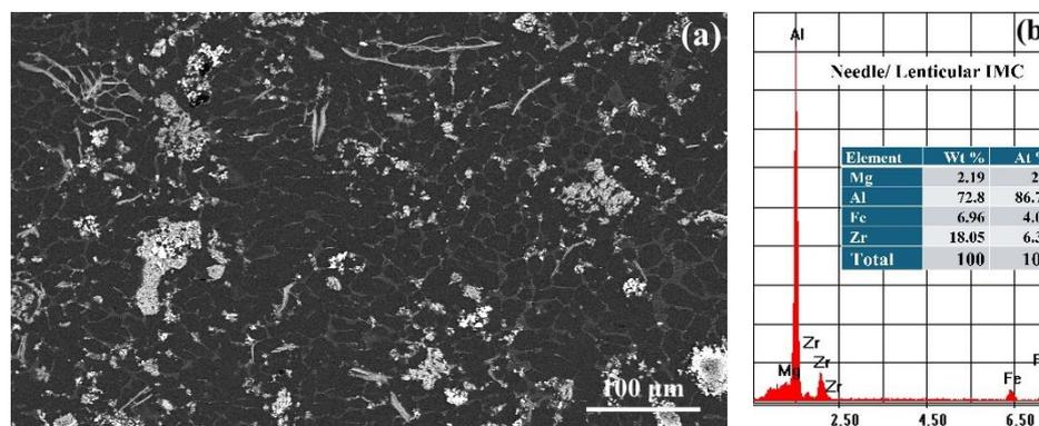
Fig. SEM image (a) and EDS analysis of AA6063/ZrB<sub>2</sub> IMC (b) with 7.5% ZrB<sub>2</sub>
