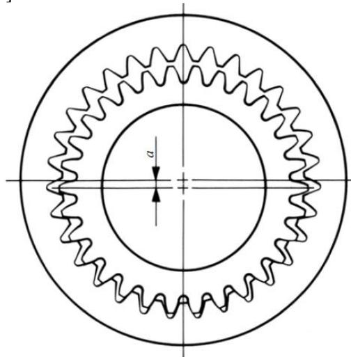
Fig. 1. Internal-external gear pair with small difference in number of teeth ( $z_2 - z_1 = 1$ ) [16].
