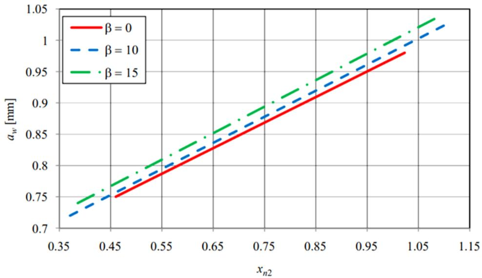
Fig. 4. The center distance,  $a_w$ , in relation to the addendum modification coefficient,  $x_{n2}$ , for the given specifications:  $z_1 = 60$ ,  $z_2 = 61$ ,  $\alpha_0 = 20^\circ$ ,  $x_{n1} = 0$ , and module  $m_n = 1$ .
