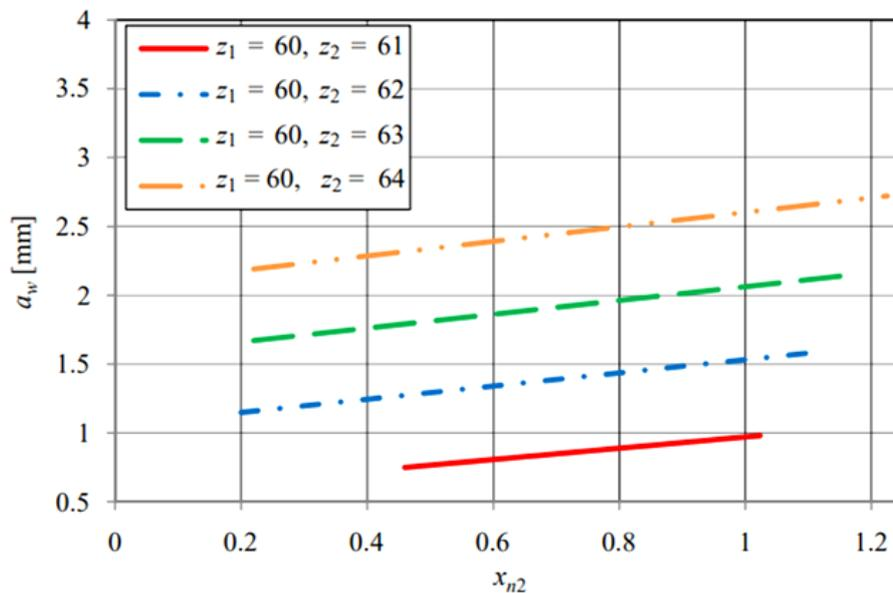
Fig. 6. The center distance,  $a_w$ , in correlation with the addendum modification coefficient,  $x_{n2}$ , under the conditions:  $\alpha_0 = 20^\circ$ ,  $\beta = 0^\circ$ ,  $x_{n1} = 0$ , and module  $m_n = 1$ .
