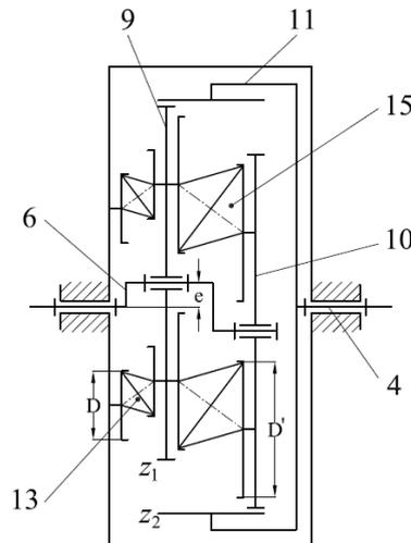
Fig. 12. Kinematics of the second planetary gear mechanism.
