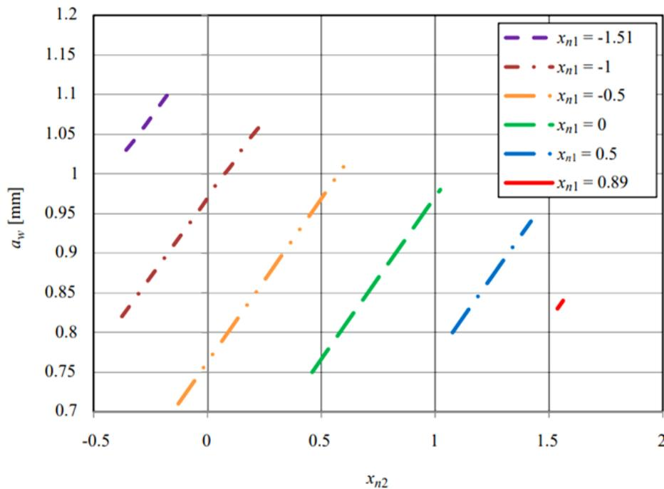
Fig. 3. The center distance,  $a_w$ , in relation to the addendum modification coefficient,  $x_{n2}$ , for the parameters:  $z_1 = 60$ ,  $z_2 = 61$ ,  $\alpha_0 = 20^\circ$ ,  $\beta = 0^\circ$ , and module  $m_n = 1$ .
