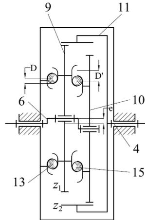
Fig. 7. Kinematics of a first planetary gear mechanism.
