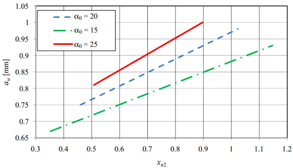
Fig. 5. The center distance,  $a_w$ , in relation to the addendum modification coefficient,  $x_{n2}$ , for the specified parameters:  $z_1 = 60$ ,  $z_2 = 61$ ,  $\beta = 0^\circ$ ,  $x_{n1} = 0$ , and module  $m_n = 1$ .
