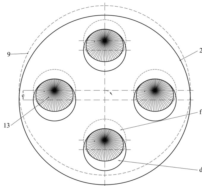
Fig. 15. Details, in frontal view, regarding the technical solution for restraining the planet gear (9) from rotating around its own axis.
