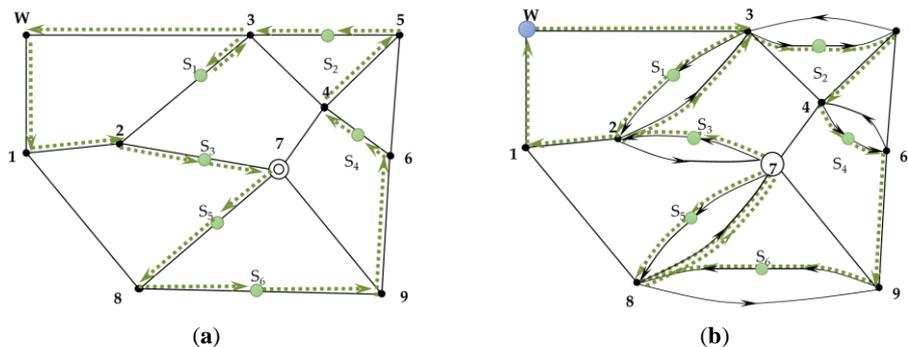
Fig. 8. Comparison of the distribution itineraries (a) initial network, without fragmentation caused by the transitway (b) network after transitway building; distribution itinerary W - S<sub>1</sub> - S<sub>2</sub> - S<sub>4</sub> - S<sub>6</sub> - S<sub>5</sub> - S<sub>3</sub> - W
