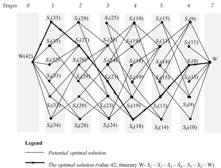
Fig. 7. Potential optimal solutions and the optimal solution for distribution itinerary
