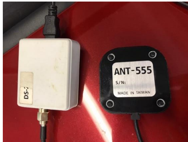
Fig. 3. The GPS Garmin device used to record the geospatial position of the tractor vehicle.
