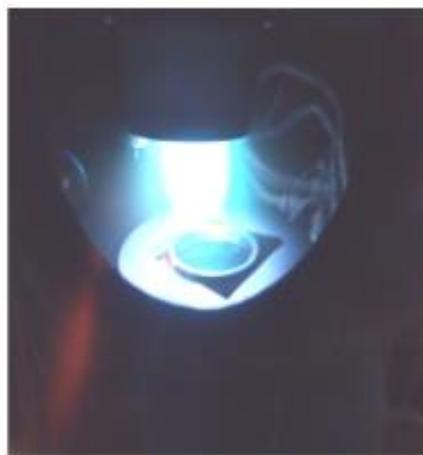
b. NiTi film sputtering on substrate
