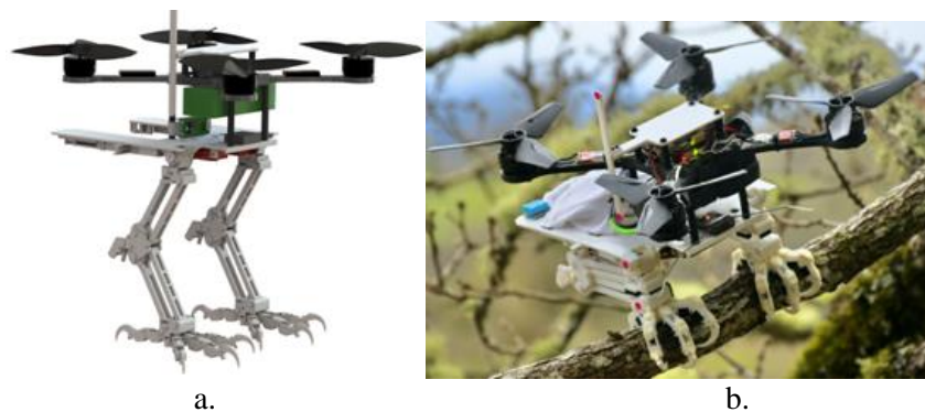
Fig. 13. Drone with claw feet (a) and this drone attachment to a tree branch (b).
