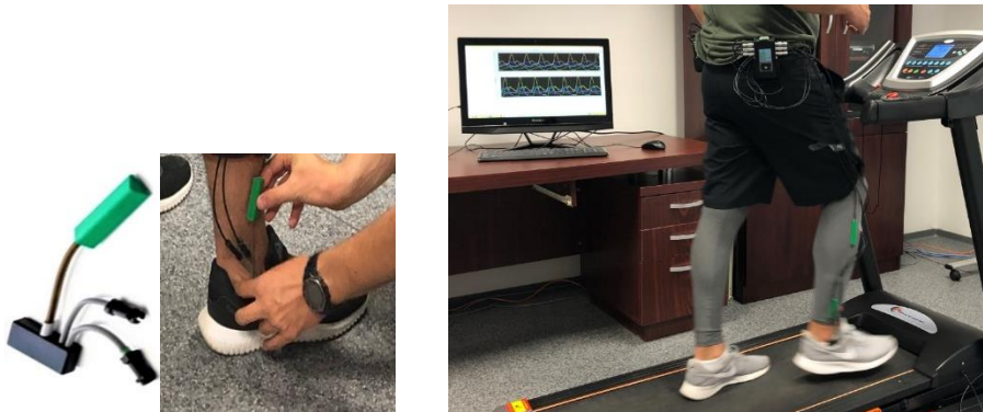
Fig. 2. (a) electrogoniometer; (b) The equipment mounted on a subject during experimental test.
