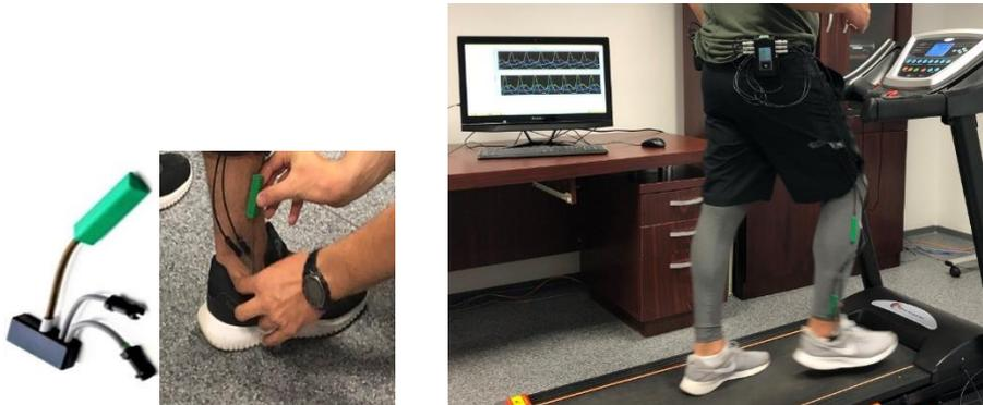
Fig. 2. (a) electrogoniometer; (b) The equipment mounted on a subject during experimental test.
