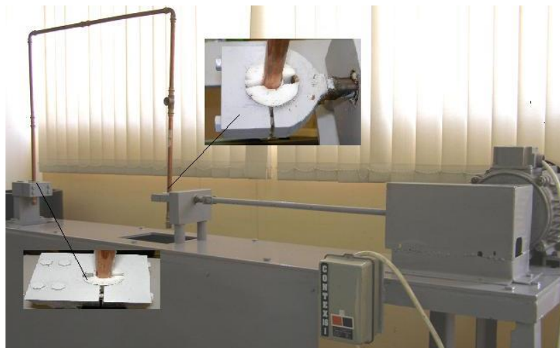
Fig. 6. Picture of the equipment for the strength test under symmetrical alternating bending loads of copper pipes joints
