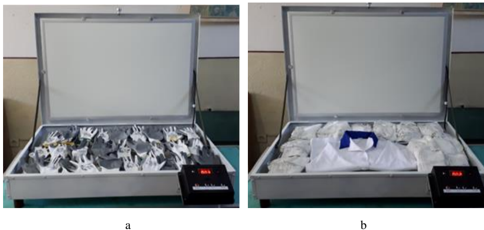
Fig. 10. (a)the equipment loaded with protective gloves; (b) equipment loaded with protective gowns.
