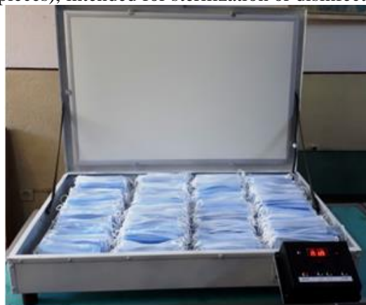
Fig. 6. The equipment loaded with the 600 sterilization masks.
