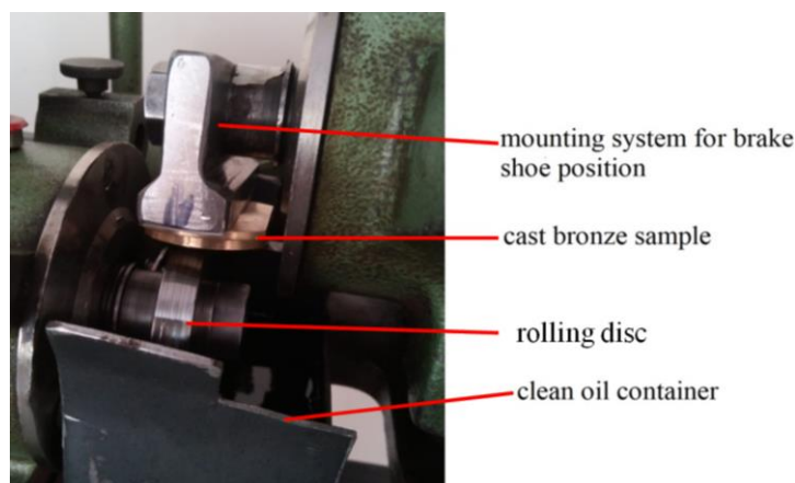
Fig. 4. Detailed aspect of the wear testing system (on Amsler type machine).
