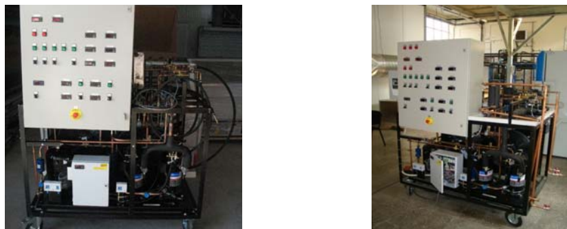
Fig. 14. Single stage R404A mechanical vapor compression refrigeration system
