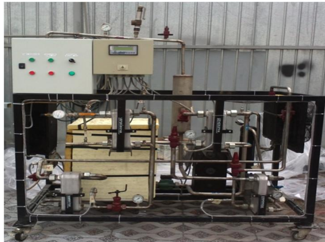
Fig. 5. Compact absorption refrigerating systems using ammonia-water solution
