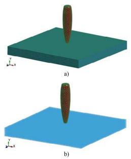
Fig. 3. Numerical analysis models (a-by FEM and b-by SPH)
