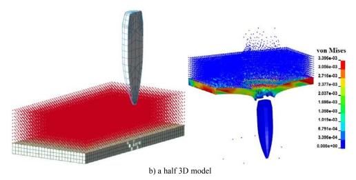
Fig. 8 The impact bullet-composite plate with two layers
