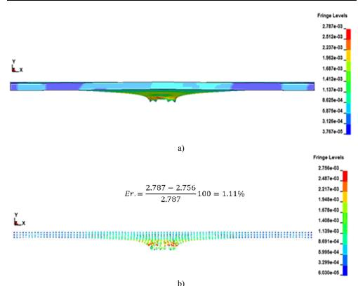
$\label{eq:b} \text{Fig. 4. The deformed state of the plate and its displacements field}$
