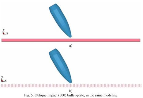
A very good concordance between results exist in the oblique impact case too. The maximum displacement occurs in Y direction (negative displacement). The error between FEM and SPH is 1.27%. The Figure 7 shows the time variation of the bullet velocity, resulting from FE (7-a) and SPH (7-b) modelling.
