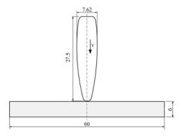
Fig. 2. Geometrical model of an impact bullet-plate
