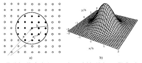
Fig. 13. Smoothing function (a-parameters, b-geometrical shape) in the space of 2D dimension
