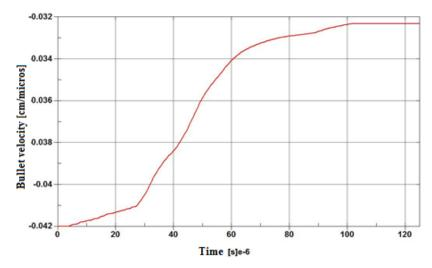
Fig. 9. Bullet velocity variation during composite plate penetration
