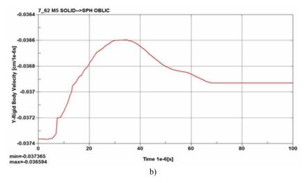
Fig. 7. Time variation of the Y-velocity of the bullet
