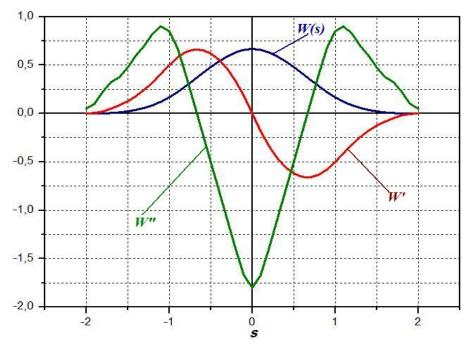
Fig. 14. The cubic B-spline smoothing function
