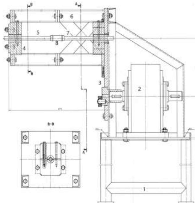
Fig. 1. Scheme of the equipment for the strength test under symmetrical alternating torsion loads of copper pipes joints:
