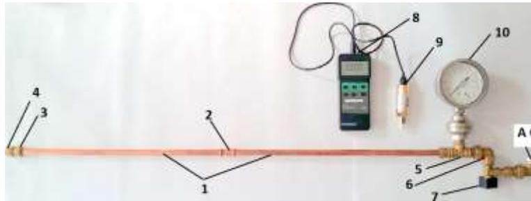
Fig. 3. Tightness testing of the specimen at internal pneumatic pressure:
