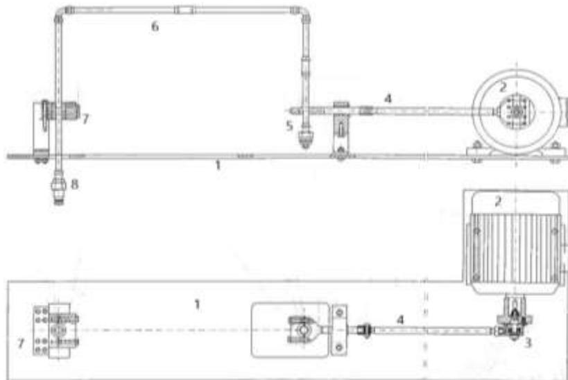
Fig. 5. Scheme of the equipment for the strength test under symmetrical alternating bending loads (vibrations) of copper pipes joints:
