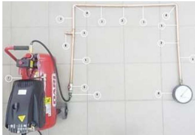
Fig. 7. Tightness testing of the U-shape specimen at internal pneumatic pressure:
