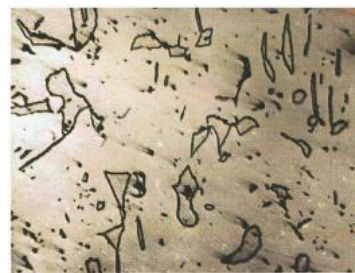
Fig. 8. Resulting microstructure after heating-up the samples according to diagram 3 Atac Nital 2%, 350 X
