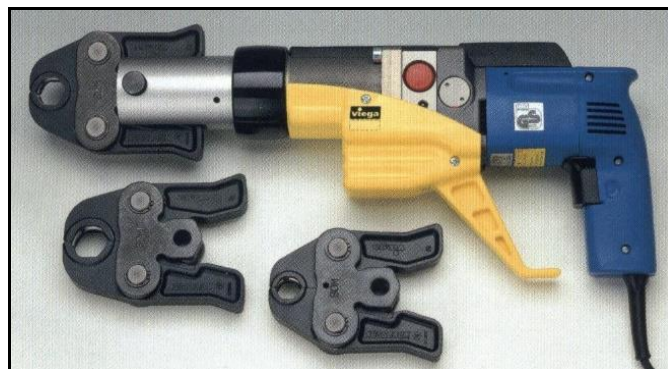
Fig. 3. Electro-hydraulic press fit device
