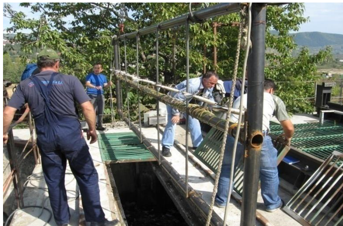
Fig. 1. Mobile frame for locating current meter.
