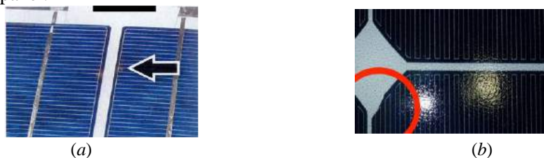
Fig. 1. Brown color traces formed during cell processing (a) and chipped PV cell (b).
