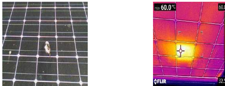
Fig. 13. Picture taken with infrared camera of a PV module with bird droppings.
