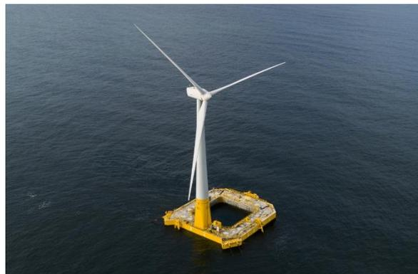
Fig. 12. Damping Pool by Ideol
