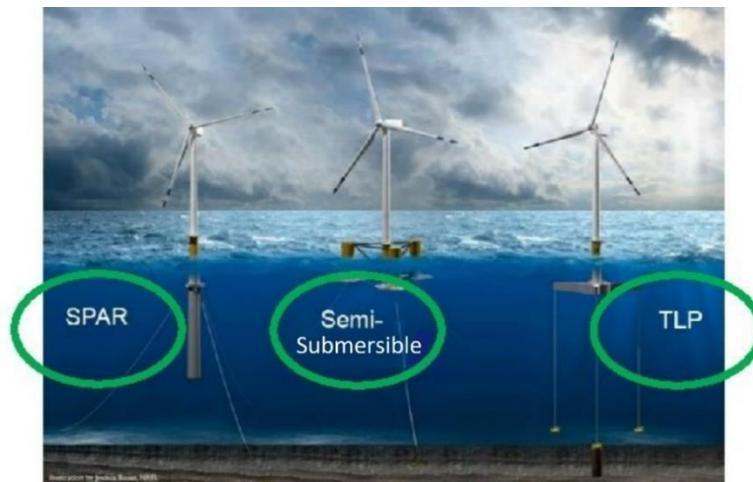
Fig. 10. Types of floating wind foundations [15]
