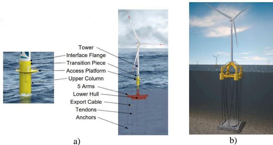
Fig. 14. a) Pelastar tension leg platform [24]; b) Gicon-SOF TLTP[25]
