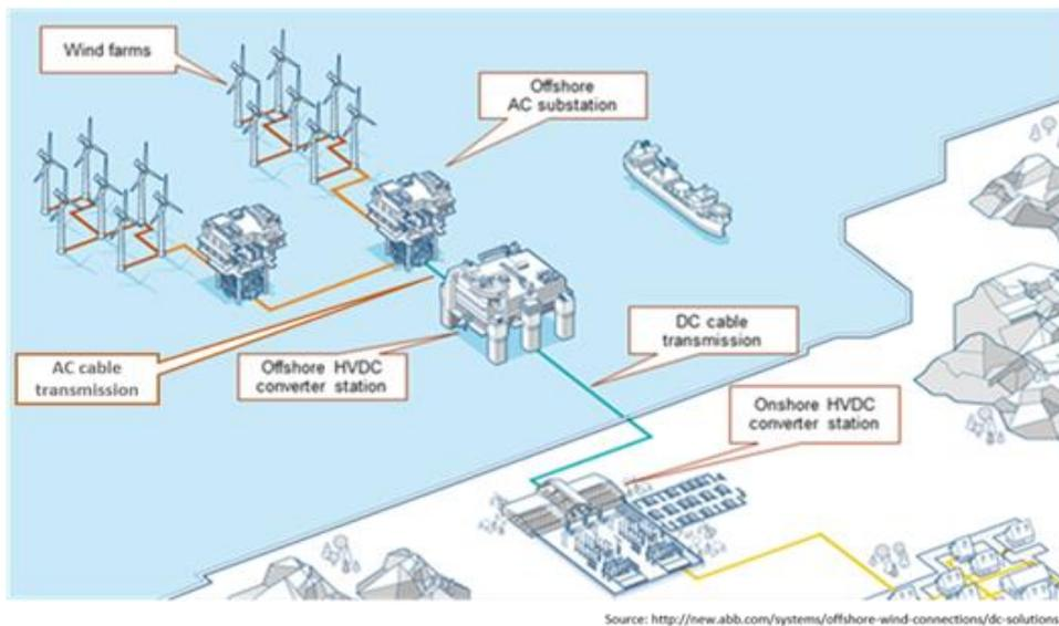
Fig. 3. Overview of offshore wind power plants [4]
