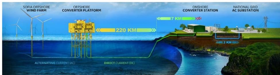
Fig. 15. Sofia offshore wind farm HVDC grid connection [26]
