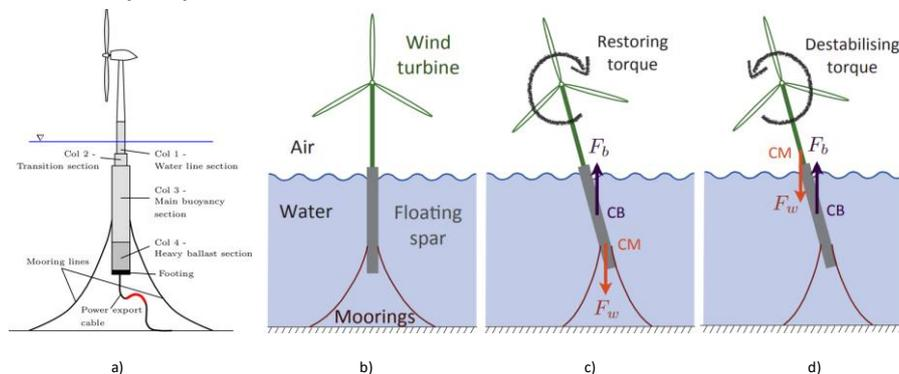
Fig. 13. a) Overview of SPAR buoy [21]; b) sketch of a spar-buoy floating WT in equilibrium; c) stable position; d) unstable position; [22]
