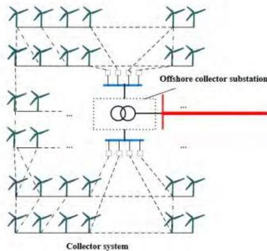
Fig. 17. Schematic diagram of a collector system [28]
