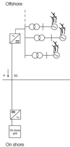
Fig. 4. HVDC for offshore wind power stations [8].
