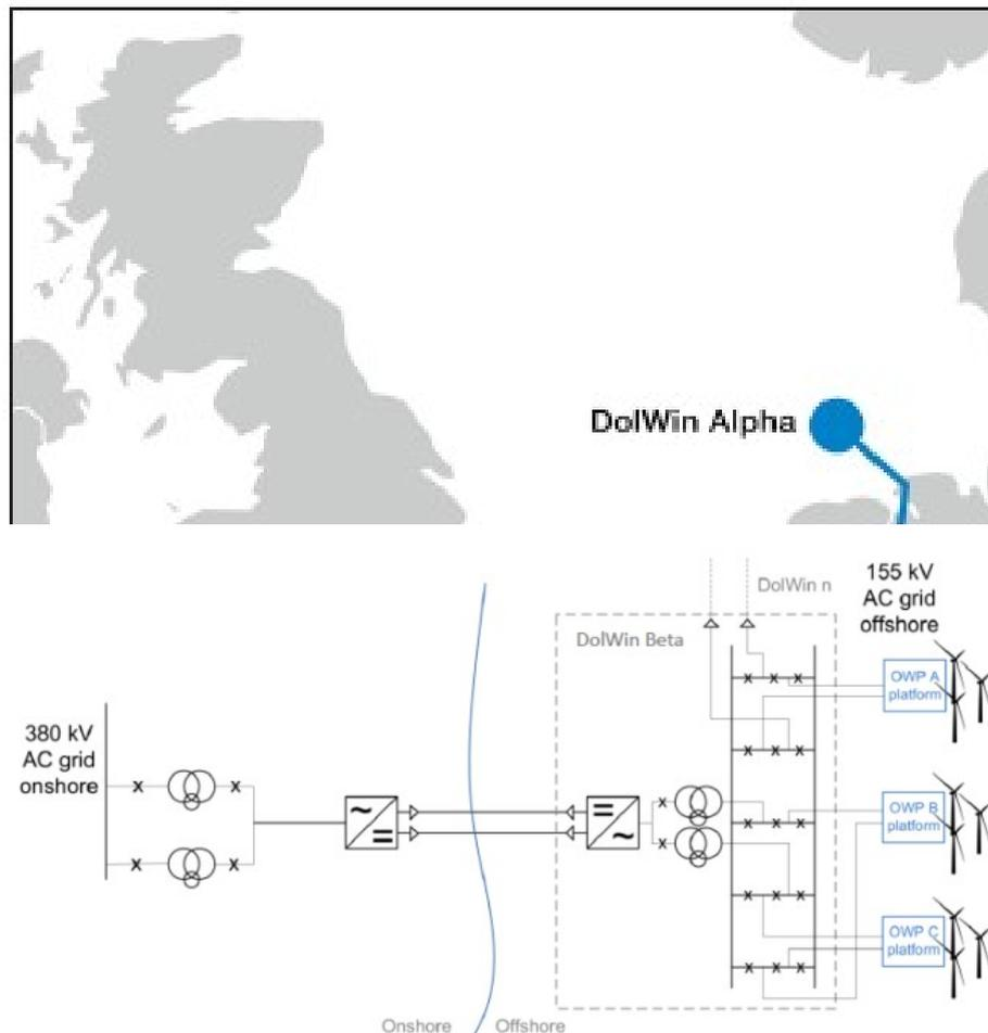
Fig. 16. HVDC connection "offshore" - "onshore" (Germany) [16].
