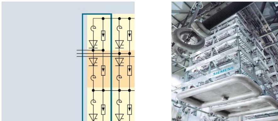
Fig. 5. 12 pulses controlled rectifier (AC-DC conversion) scheme and picture [7].
