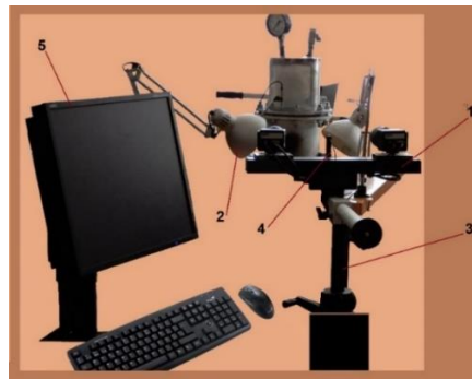
Fig. 5. ARAMIS system components: Schneider two-chamber sensor (1); two LED lamps (2), stand for supporting and fixing the sensor (3); camera shutter system and image recording control (4); High-performance PC (5) operating under the GOM Linux 7 system and specialized software version 6.1 [26; 27].
