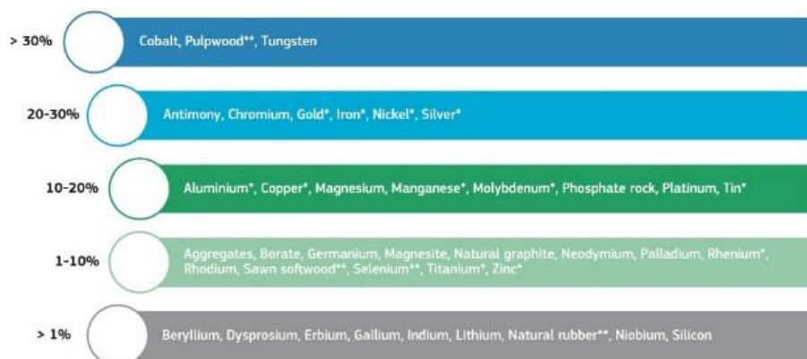
Fig. 5. End-of-life recycling entry rates (EOL-RIR) for some metals, [17].
