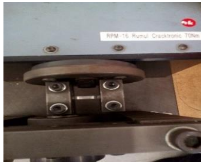
Fig. 7. Positioning of eprouvette in the fatigue testing machine.
