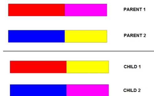
Fig. 2. A crossover with two parents and two offsprings (childs) with one cutting point.
