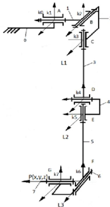
Fig. 2. Kinematic structure of the robotic arm.
