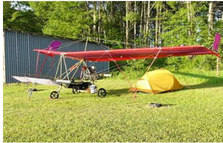
Fig. 1. a. Pterodactyl Ascender ultralight aircraft, mass 57 kg.
