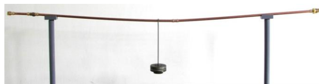
Fig. 6. Picture of the device for the static bending testing of the copper pipes assemblies
