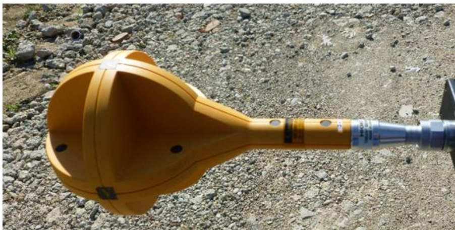
Fig. 1. Magnetic field tester measurement test Hioki FT3470-50, [22].
