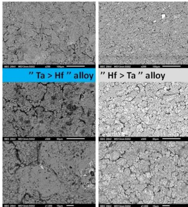
Fig. 11. Imaging of the gold-coated oxidized surfaces of both alloys: "Hf > Ta" alloy (left) and "Hf > Ta" alloy (right); general view ( $\times 250$ , top) and two more detailed views ( $\times 500$ , middle) and ( $\times 1000$ , bottom); WF-SEM in BSE mode.
