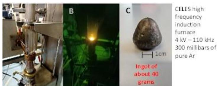
Fig. 1. The hottest part of the furnace before (A) and during melting (B); one of the obtained ingots (C).
