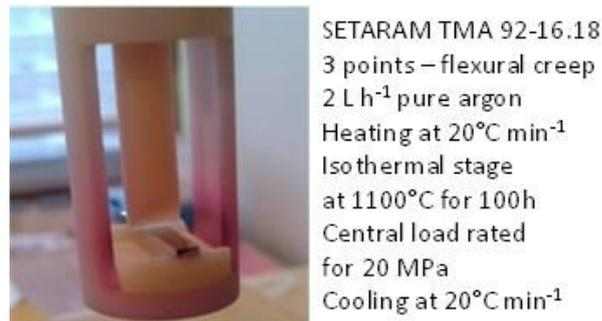
Fig. 3. The creep sample before introduction in the furnace and the application of the constant force.
