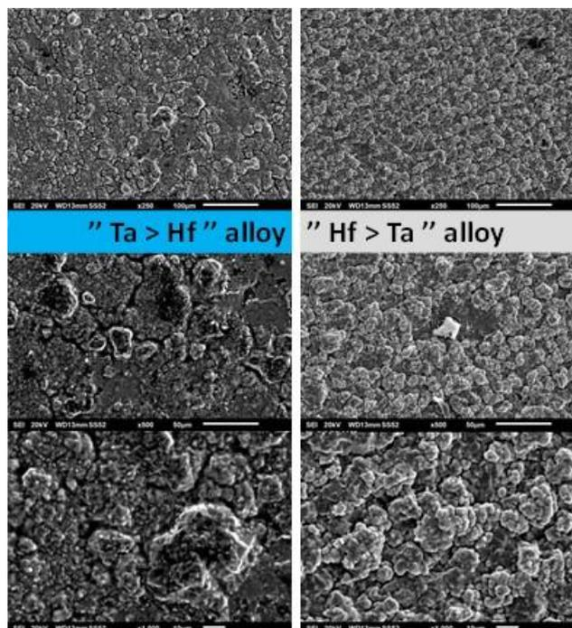
Fig. 10. Imaging of the gold-coated oxidized surfaces of both alloys: “Ta > Hf” alloy (left) and “Hf > Ta” alloy (right); general view ( $\times 250$ , top) and two more detailed views ( $\times 500$ , middle) and ( $\times 1000$ , bottom); WF-SEM in SE mode.
