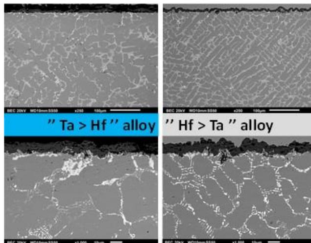
Fig. 12. BSE imaging (WF-SEM) of the oxidized surfaces and subsurfaces of the two alloys "Ta > Hf" (left) and "Hf > Ta" (right); general view ( $\times 250$ , top) and detailed view ( $\times 1000$ , bottom); WF-SEM in BSE mode.
