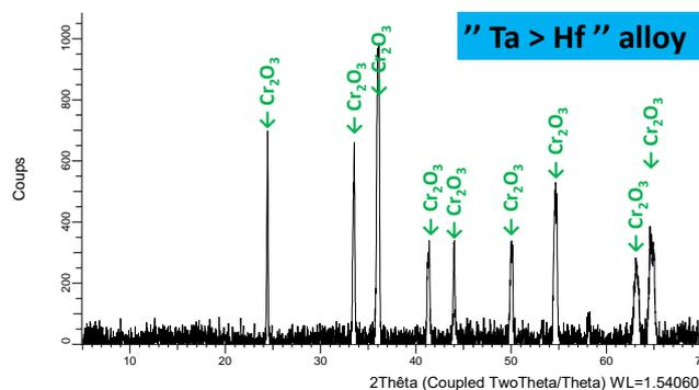
Fig. 8. Diffractogram acquired on the oxidized surface of the “Ta > Hf” alloy.
