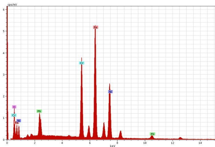
Fig. 4. The EDS spectrum and quantitative composition of the layer formed on Incoloy 800 , exposure time 30 days,  $t=260^{\circ}\text{C}$ ,  $p=5.1$  MPa,  $\text{pH}=9.5$  in the presence of 300 mg/L PbO
