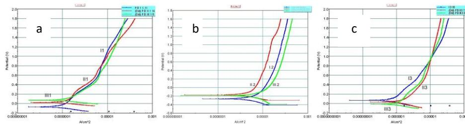
Fig. 5. Potentiodynamic polarisation graphs of the oxides films formed on Incoloy 800,  $t=260^{\circ}\text{C}$ ,  $p=5.1\text{ MPa}$ ,  $\text{pH}=9.5$  in the presence of PbO: 100 mg/L (a), 200 mg/L (b) and 300 mg/L (c), exposure times 10 days (a), 20 days (b) and 30 days (c)
