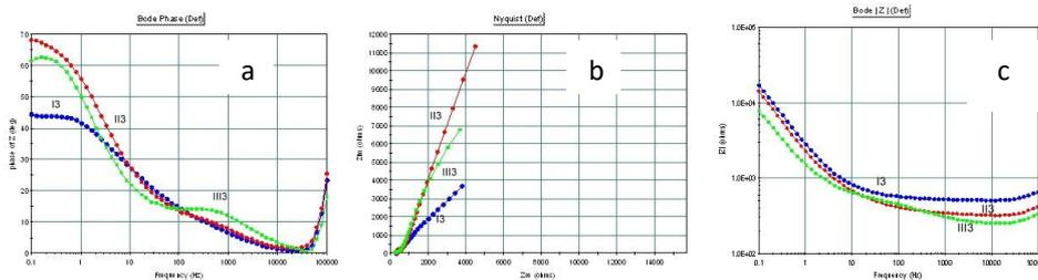
Fig. 6. Phase angle (a), Nyquist (b) and Bode (c) curves for Incoloy 800,  $t=260^{\circ}\text{C}$ ,  $p=5.1\text{ MPa}$ ,  $\text{pH}=9.5$  in the presence of PbO: 100 mg/L (I.3.), 200 mg/L (II.3) and 300 mg/L (III.3), exposure time 30 days
