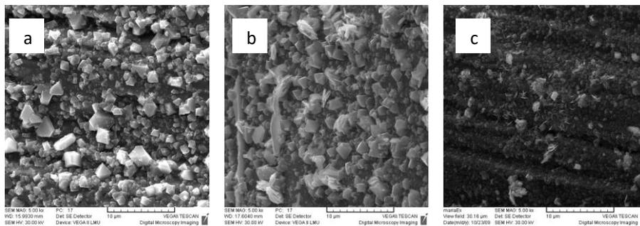
Fig. 3. The SEM morphology of the oxide films formed on Incoloy 800, exposure time 30 days,  $t=260^{\circ}\text{C}$ ,  $p=5.1$  MPa,  $\text{pH}=9.5$  in the presence of PbO: 100 mg/L (a), 200 mg/L (b) and 300 mg/L (c)
