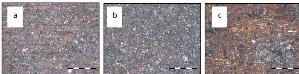
Fig. 1. The morphology of the oxides films on Incoloy 800, exposure time 30 days,  $t=260^{\circ}\text{C}$ ,  $p=5.1\text{ MPa}$ ,  $\text{pH}=9.5$ , in PbO presence: 100 mg/L (a), 200 mg/L (b) and 300 mg/L (c)
