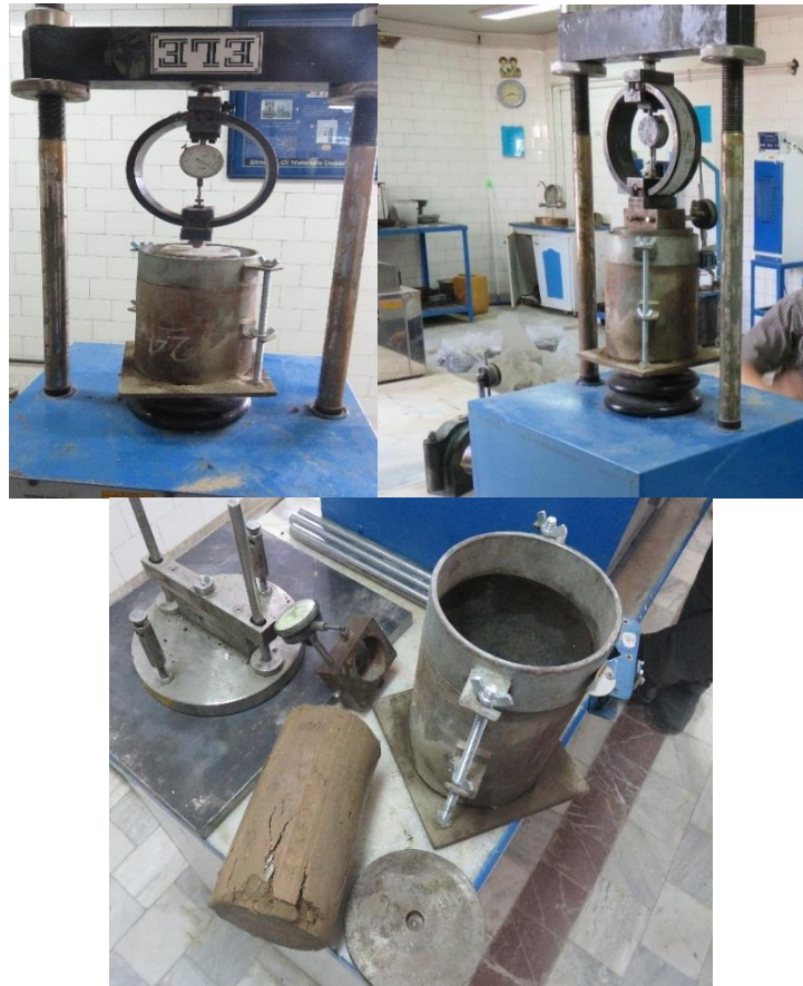
Fig. 3. Uniaxial compressive strength test.
