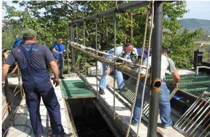
Fig. 1. Mobile frame for locating current meter.
