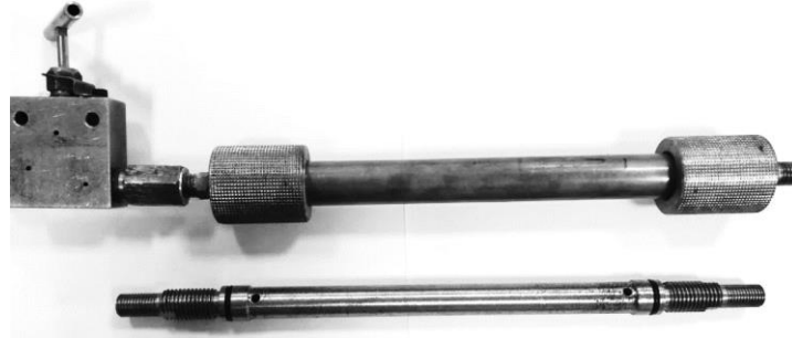
Fig. 7. Experimental stand used to determine the bursting pressure for Copper pipes with volumetric surface defect.
