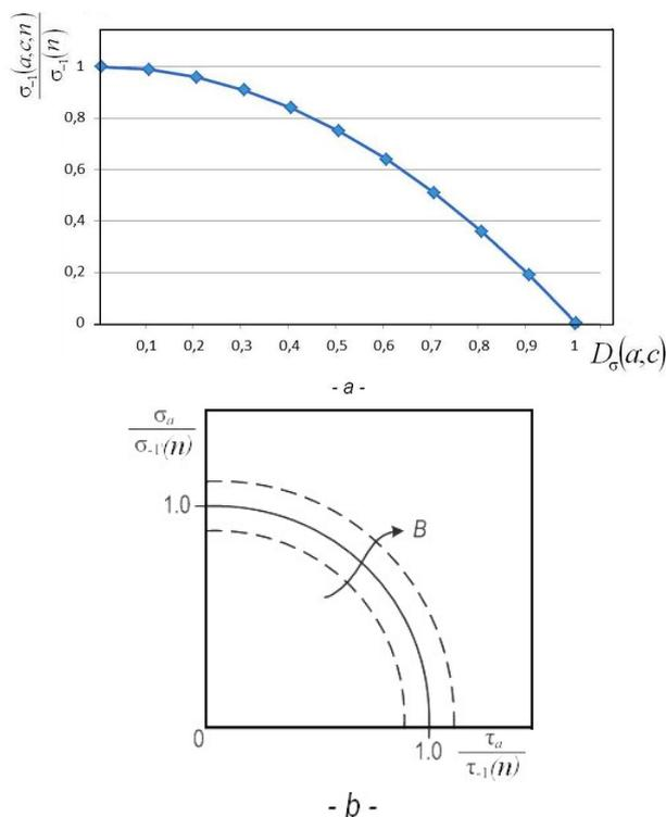
Fig. 3. a - Fatigue strength versus deterioration due to crack, according to the first eq. (17) for  $P_{cr}(0) = 1$  and a given value of  $k$ ; b - diagram of the superposition of cyclic loading with a normal stress and a shear stress, according to relation (19).
